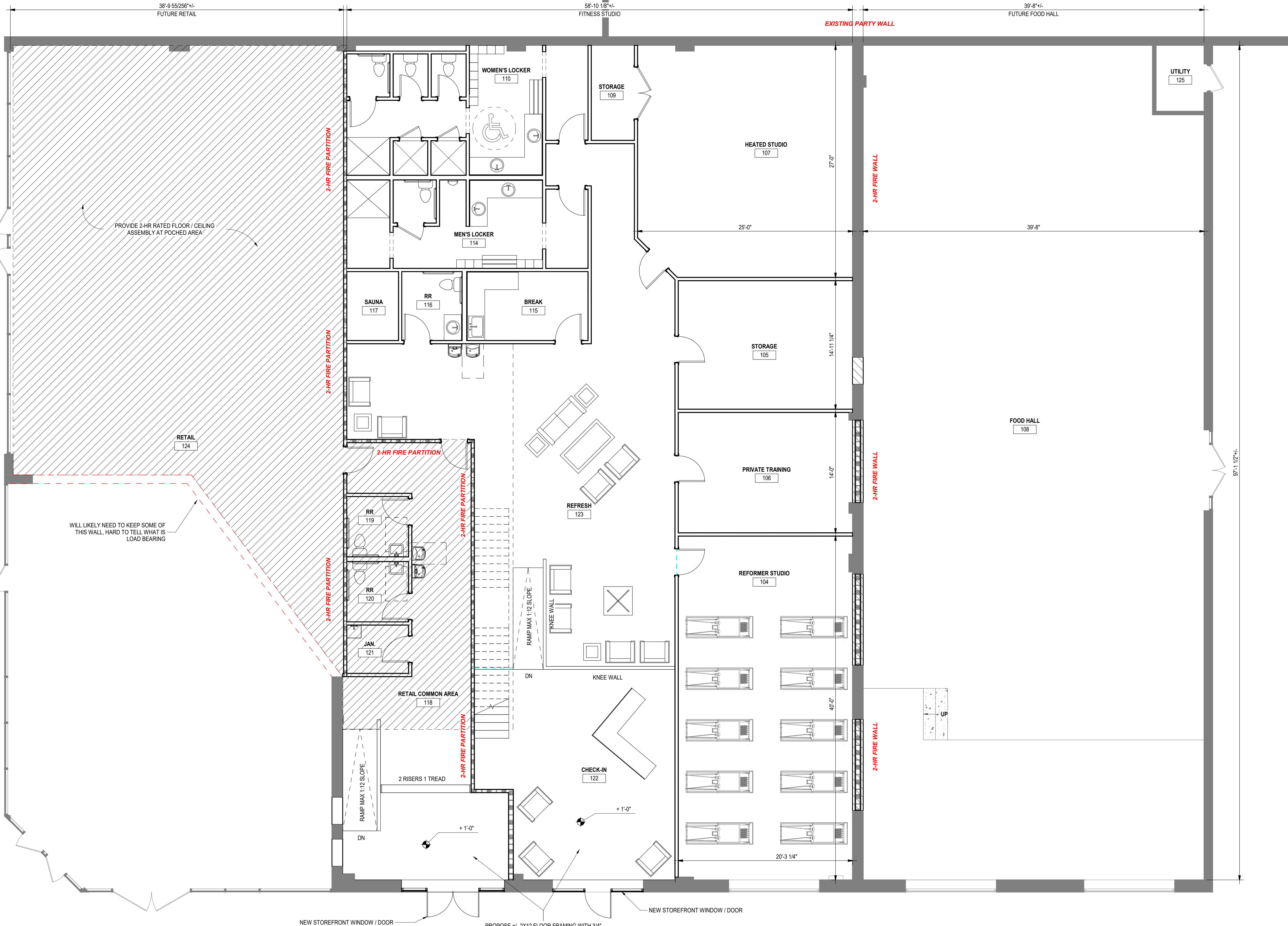
1 CONSTRUCTION PLAN - LEVEL 01 A-101 | 3/16\"/>
