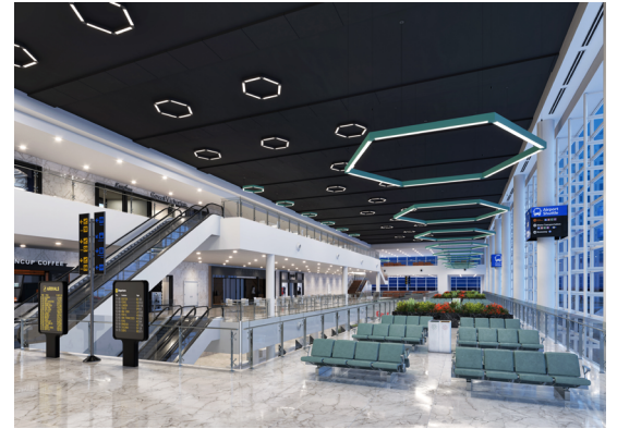
Large Hexagon - S4PDMP CPP 24FT 6120NC 6ea 4' Sections with 6ea 120° corners Small Hexagon - S4SDMP CPP 12FT 6120NC 6ea 2' Sections with 6ea 120° Corners
