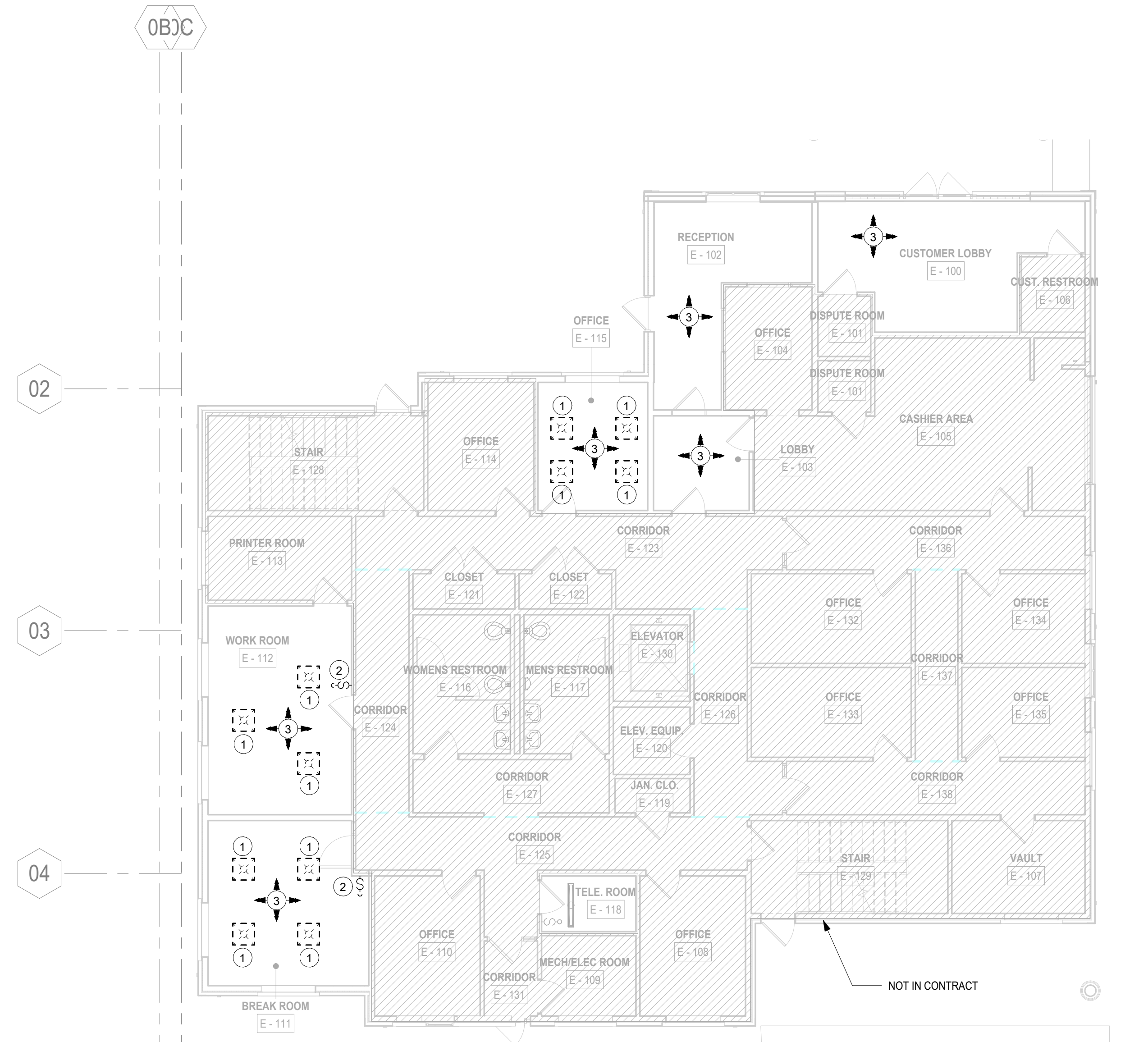
1 FIRST FLOOR LIGHTING PLAN - DEMOLITION SCALE: 1/8" = 1'-0"
